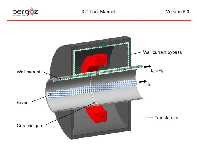
The transformer "sees" all currents passing through its aperture, i.e. beam current  $I_b$  and high frequency components of wall current  $I_w$ . Since these two currents cancel each other, only the beam current components whose corresponding wall current is diverted over the wall current bypass and the high frequency resonances are visible to the transformer. Only these currents induce a magnetic flux in its core.
