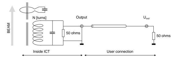
The ICT is a fast capacitively shorted transformer coupled to a slow readout transformer in a common magnetic circuit<sup>1</sup>.
