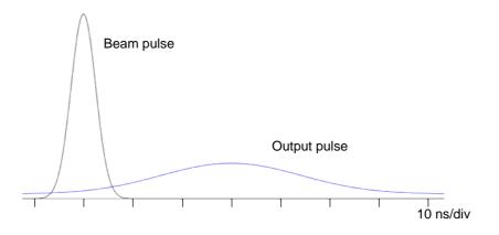
The sensitivity of the Integrating Current Transformer is also called transfer impedance. It depends on the ICT model. It is expressed in terms of the integral of the output pulse voltage as a function of the input pulse charge, therefore in Vs/C, or  $\Omega$ .
