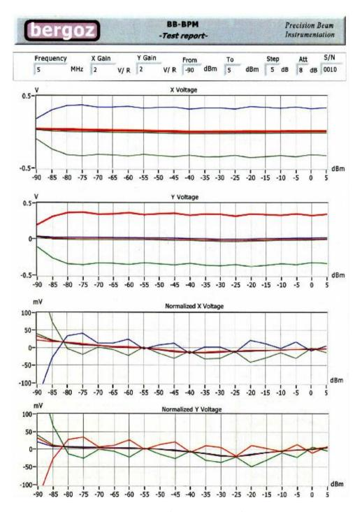
Note: X and Y signal displays are limited to ~1 kHz (10 kHz on option) by the virtual instrument LabVIEW.
