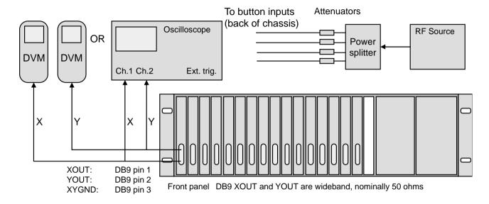
To display X and Y signals, either use two DVMs, or an oscilloscope. The front-panel DB9 outputs are 50 ohms nominal impedance. Attach the equipment together as shown above.
