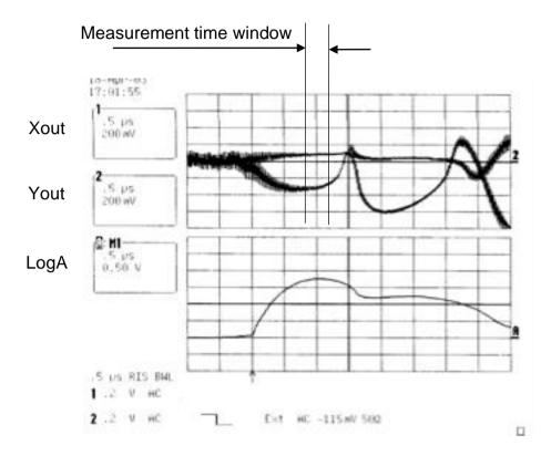
Observe the Xout and Yout signals represent X/Y positions for  $\sim 500$  ns about LogA pulse apex.
