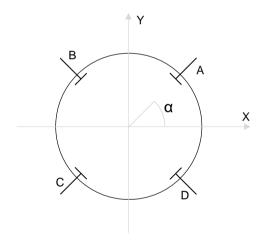
Note: Pickups with larger f, such as stripline and shoebox, have higher coupling impedance (they collect more signal from the beam) but lower sensitivity to beam displacement. Pickup sensitivity increases with f as  $\sin(f/2) / f^1$ .
