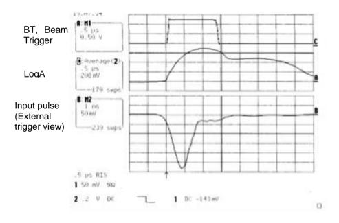
Observe the Beam Trigger BT rising ~1 us before the apex of LogA.
